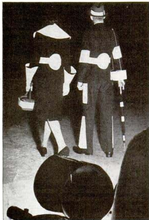
Special shades are fitted over the rear lights of motorcycles used to lead buses and streetcars in Manchester, England, in fog or blackout
